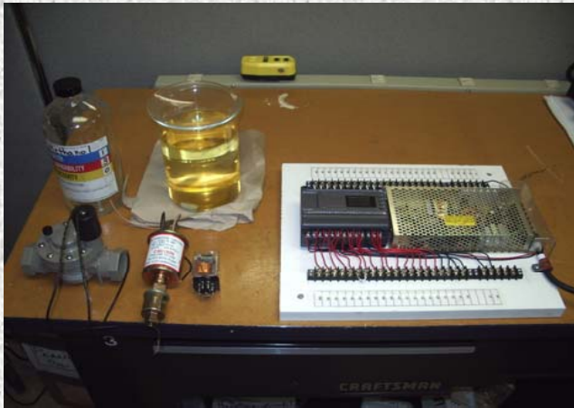
Various Chemicals and Components used in the process (clockwise from top left (Methanol, finished biodiesel, PLC Board, Actuator, Diesel Pump, Sprinkler Valve)
