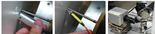
Fig. 2 Left to right, IR LED, Fiber Optic, and Xenon Flash methods.
