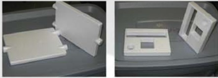
Two Different Types of EPS Foam Used Throughout Testing
