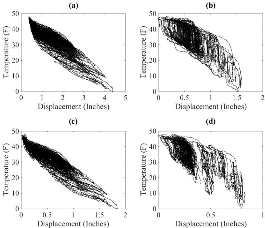
**Figure 12: Measured Displacements: a) Pier 5: Relative Displacement at Expansion Joint, b) Pier 7: Relative Displacement at Expansion Joint, c) Pier 5: Absolute Displacement at Bearing, and d) Pier 7: Absolute Displacement at Bearing**
