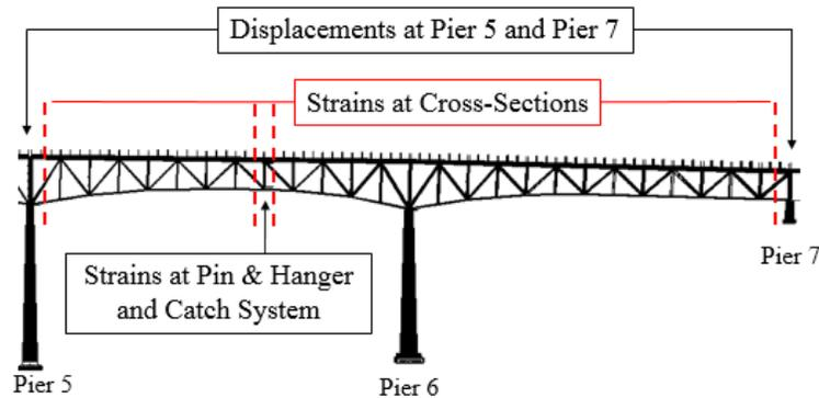
**Figure 7: Instrumentation Plan Overview**
