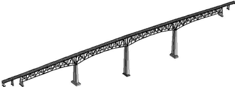
**Figure 5: Finite Element Model of Hurricane Bridge**
