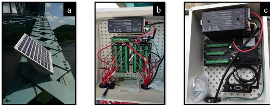
**Figure 9: Monitoring Equipment: a) Solar Panel, b) DAQ Box, c) Ground Station**
