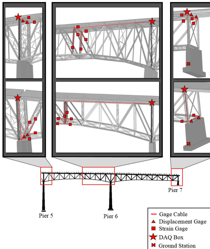
**Figure 8: Detailed Instrumentation Plan**
