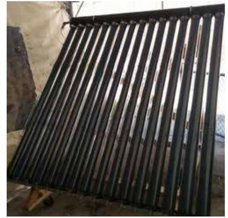
An evacuated-tube water heater, which is being tested for the elephant hut prototype.
